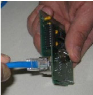
FIGURE 1 - 7 Insert the card
