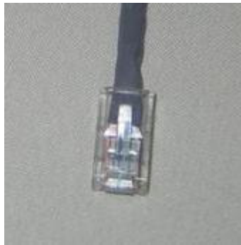
FIGURE 1.3 No Hood Cable
