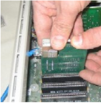
FIGURE 1 - 13 Seat the card
