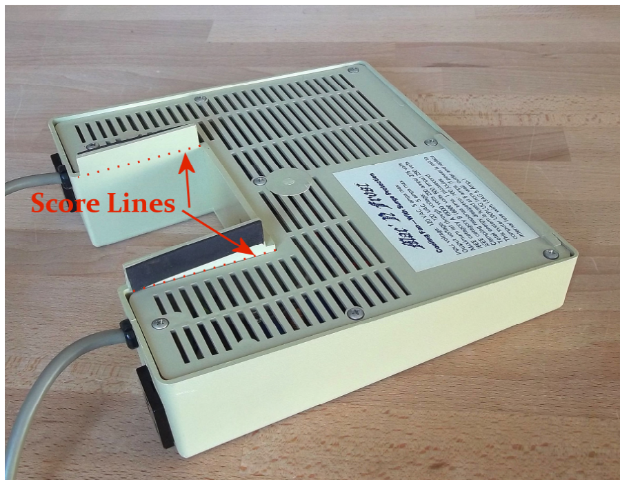
Figure 2. Score lines for removal of fins.
