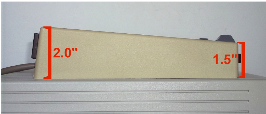
Figure 4. Unit in its upright position after removal of the fins & ridge. Notice that the bottom should be flush with the surface it rests upon.
