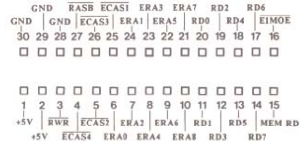
Figure C-10 Expansion memory connector
