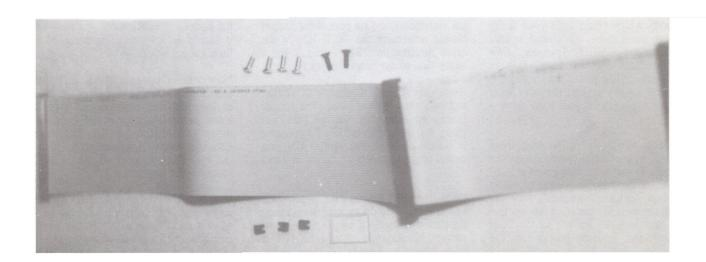
Photo 2 - Top to Bottom: Mounting Screws, Internal SCSI Cable and Jumper Blocks
