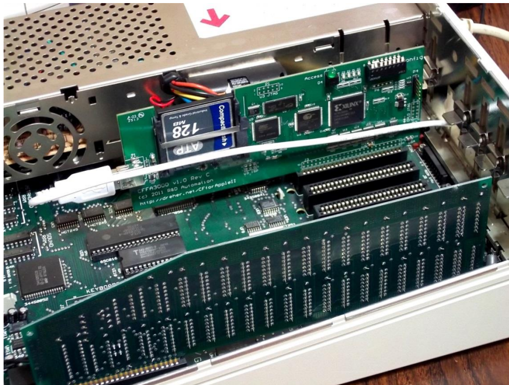
Figure 1.1. CFFA3000 card installed in slot 2 with USB extension cable attached and threaded out through the back of the IIGS case.
