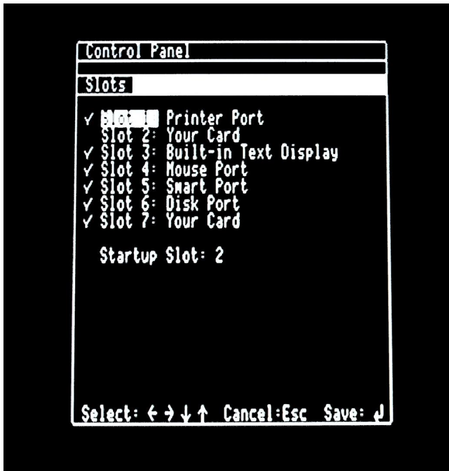
Figure 1.5. Control Panel | Slots showing Slot 2 and Slot 7 set to “Your Card” and Startup Slot set to “2”.
