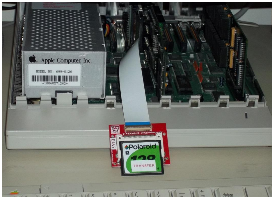
The MicroDrive Turbo installed in my IIGS with one CompactFlash card accessible via a CF Extender.
