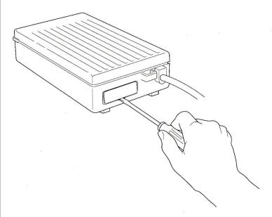
3. Plug the second drive's cable into the connector on the back of the first drive and tighten the retaining screws.
