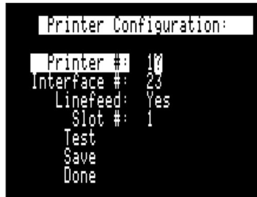
The Screen display will appear as in Figure 3.(11)-3. You will be able to completely configure and test your printer and interface in this menu. This page will take you through the process step by step:
