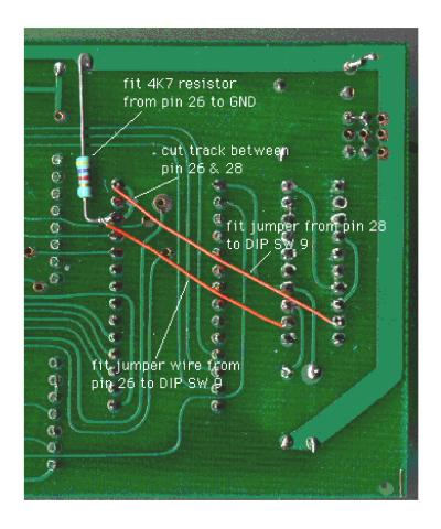
Should you wish to remove the modification simply remove the resistor and the jumpers and install a new jumper between pin 26 and pin 28 of the Textool instead of repairing the cut track.
