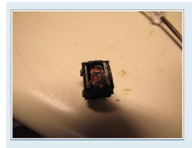
11. Replace the cover and press it into place. It will only go on one way - make sure the contact holes line up with the contacts. Ensure the tabs have locked into place. Test your switch with your continuity tester - the switch should be on when the plunger is pressed.
