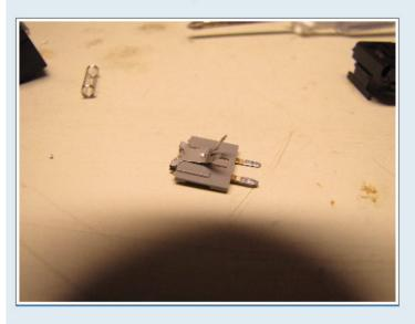
It consists of a pair of metal plates and a bent piece of metal similar to the tactility spring. When the plunger moves down, this actuator pushes down on a plastic tab underneath that in turn presses together the contact plates, completing the circuit.
