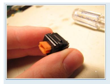
See the "T"-shaped tap on the side of the keyswitch? Use a thumbnail to pull away this one and the other one on the other side while applying pressure to the protruding contacts of the switch. This will make the assembly come apart:
