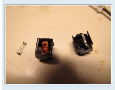
There are four important parts to the keyswitch: the spring, the tactility spring, the plunger, and the contact assembly.
