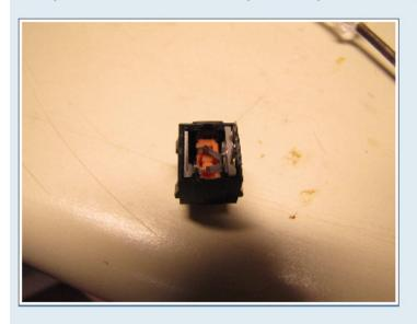
Note that the metal arms should be nearly touching. Otherwise the metal actuator hasn't been bent enough. Insert the spring into the middle:
