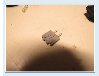
10. Replace the metal actuator, and then place all components into the upper half of the keyswitch assembly like shown:
