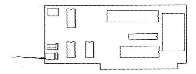
The transducer itself should be placed near enough to the controller to operate. This can be as far away as 6 or 8 feet if the transducer is aimed directly at the pickup inside the controller box. After installing the H.O. with the BSR interface attached, you can type in the program below to test the positioning of the transducer. When the program is running, you should see the red light on the controller flashing on and off.
