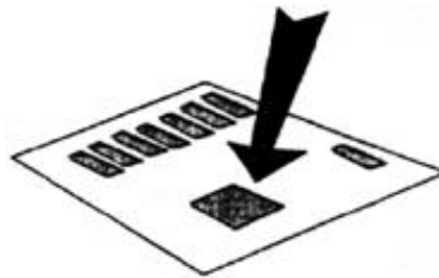
Fig. 5. Once the ZipGS product is installed into the socket press firmly to insure good contact BE CAREFUL NOT TO BEND ANY PINS!
