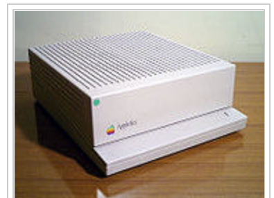
The Apple IIGS, the most powerful Apple II, featuring a true 16-bit CPU, 4096 colors, Ensoniq synthesizer, a Mac-like GUI and a mouse.
