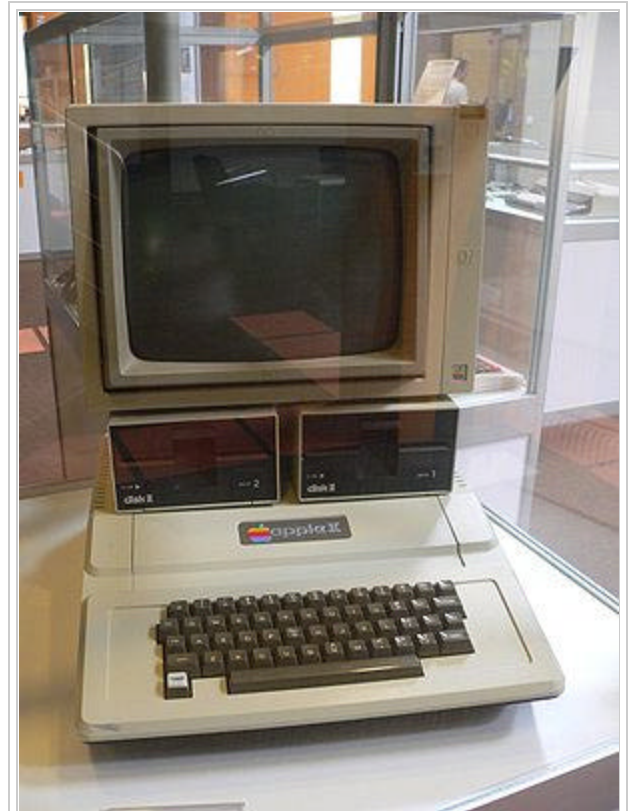
The 1977 Apple II, shown here with twin floppy disk drives and a monitor. The Apple II featured an integrated keyboard, sound, a plastic case, and eight internal expansion slots.
