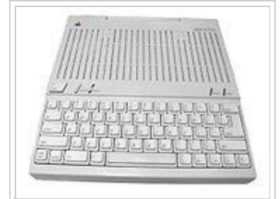
The Apple IIc Plus, an 8-bit revision of the original portable but with faster CPU, 3½-inch floppy and built-in power supply. It was the last of the Apple II line.
