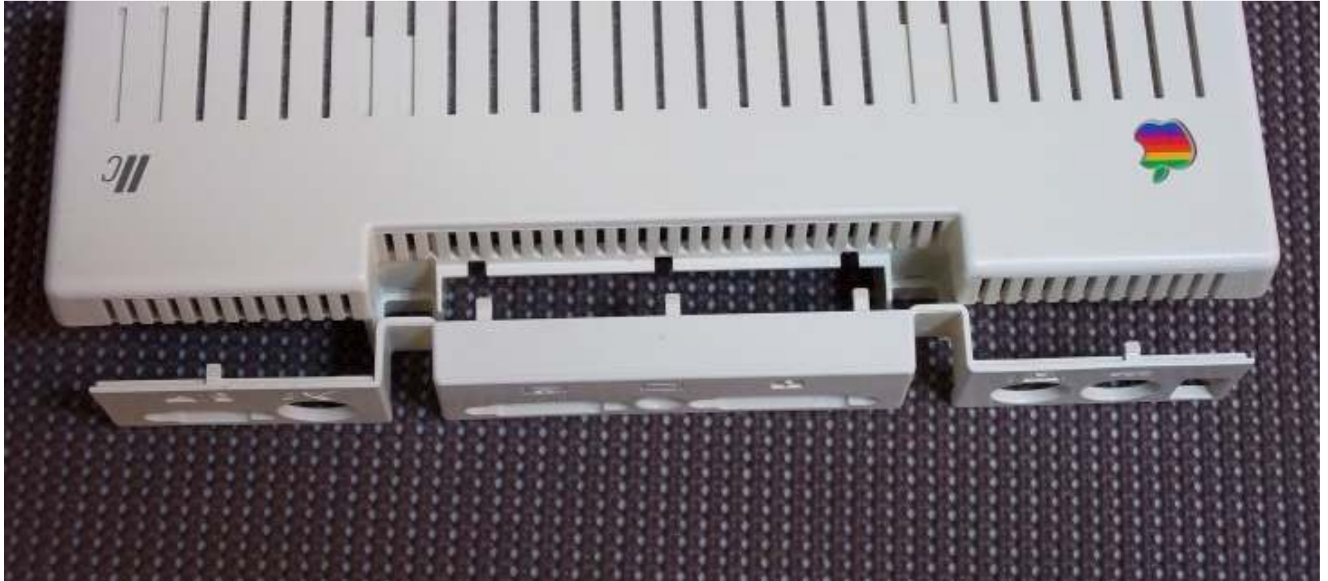
Figure 7. Top view of the separation of the backplate from the top of the Apple IIc case.
