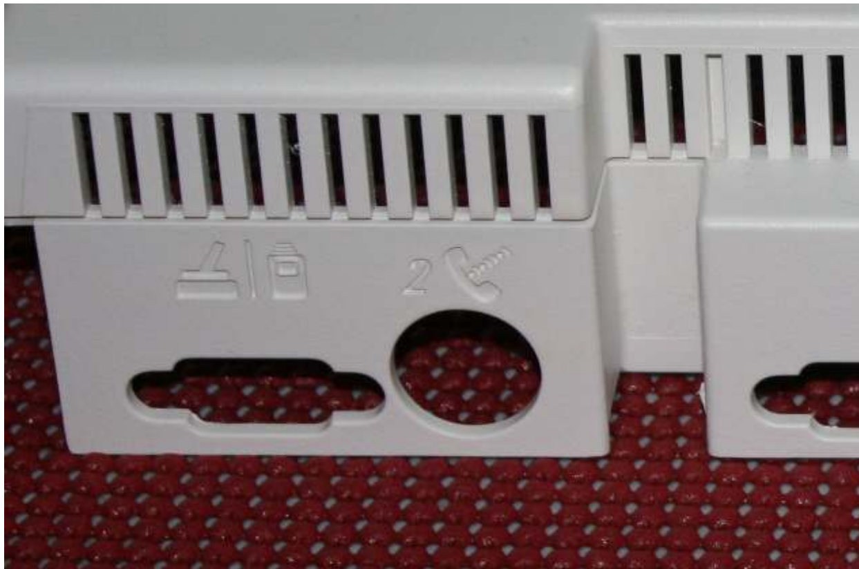
Figure 1. Left portion of the back plate from a Type 1 Apple IIc case.
